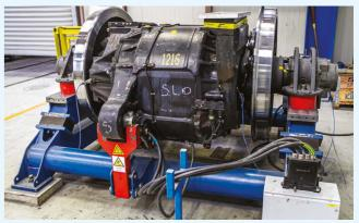
Four years after the previous wheels were replaced, the 541 (Siemens Taurus) needed new wheels. Our shops did their first shrink fitting of monobloc wheels back in 2019, which was the first round of replacing the wheels on the freight locomotives operated by SŽ – Tovorni promet. Currently, our workshop is busy with the second round of wheel replacement for Tovorni promet, which was launched at the end of 2023, starting off with the 541-017.
