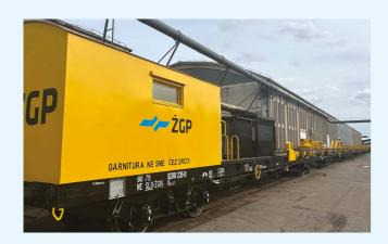
At the end of 2023, a Robel 40.61 – SILAD long-rail train entered our workshop for an overhaul from the Slovene rail engineering and construction company Železniško gradbeno podjetje (ŽGP). The train consists of nine four-axle flat wagons with a total length of 178.2 m and is designed to transport, load and unload rails up to 120 m long.
