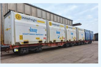
At the Dobova centre, we perform overhauls in accordance with the VPI for 14 international companies, one of which is Innofreight. The company is renowned for its innovative solutions in freight transport, specifically the Sggrrs series of modular flat wagons. These wagons can be fitted with various superstructures to accommodate different types of cargo.
